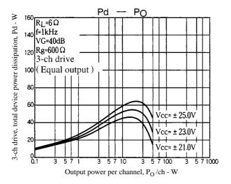
The total device power dissipation when hybrid IC's  $V_{CC} = \pm 23V$  and  $R_L = 6\Omega$ , for a continuous sine wave signal, is a maximum of 55W, as is in Pd-P<sub>O</sub> graph.
